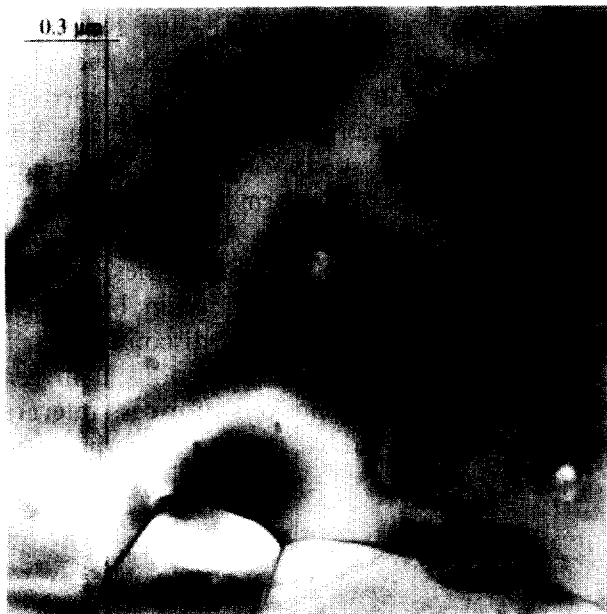
Fig. 1. Microstructure of \text{Al}_2\text{O}_3 -SiC nanocomposite: SiC particles \leq 150 nm situated in intragranular positions; microcracks indicated by arrows (TEM-BF image; material A).
